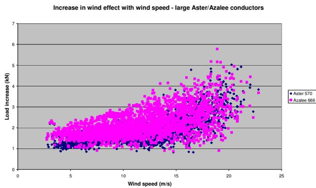
Fig. 6.2 Comparison of wind effects on large Aster and Azalee conductors
