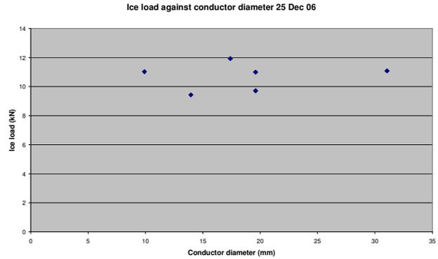
Fig. 4.1 Conductor rime ice load against conductor diameter (Dec 2006)
