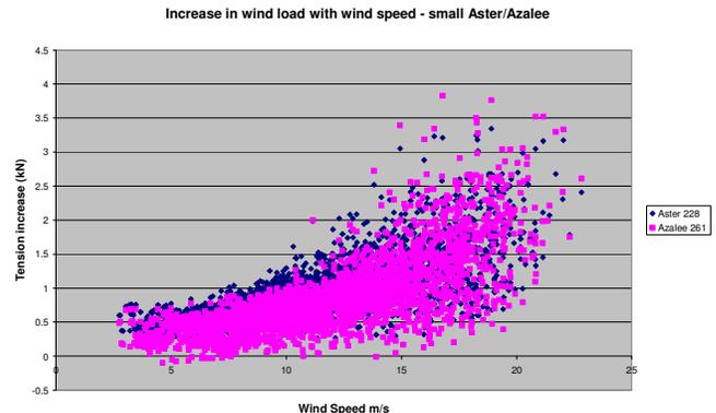
Fig. 6.1 Comparison of wind effects on small Aster and Azalee conductors
