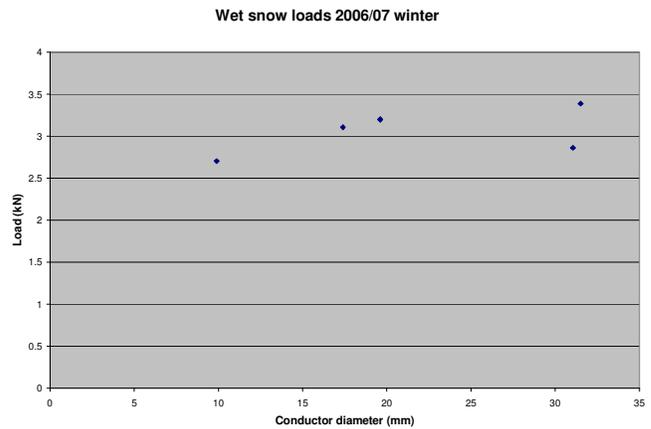
Fig. 5.1 Mean wet snow loads against conductor diameter for winter 2006/07
