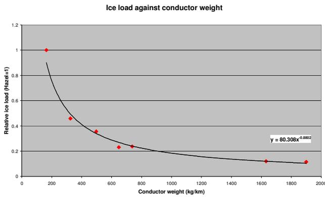
Fig.4.3 Ice load weight against conductor weight (kg/m) normalised to Hazel.
