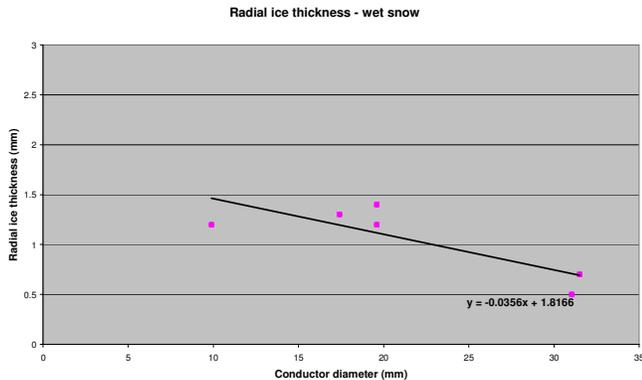
Fig. 5.3 Wet snow radial ice thickness against conductor diameter
