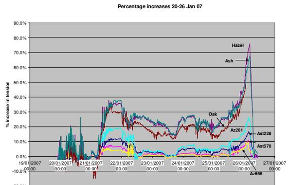
Fig.4.2 Percentage increases in tension for all conductors in January, 2007
