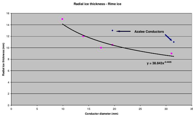
Fig. 4.4 Radial ice thickness against conductor diameter
