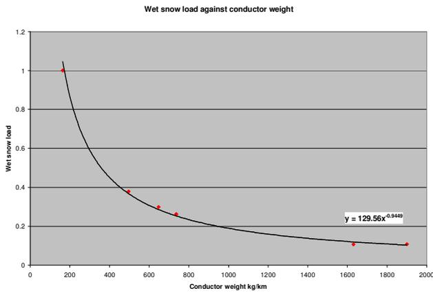
Fig. 5.2 Variation of wet snow load with conductor weight (normalized to Hazel)
