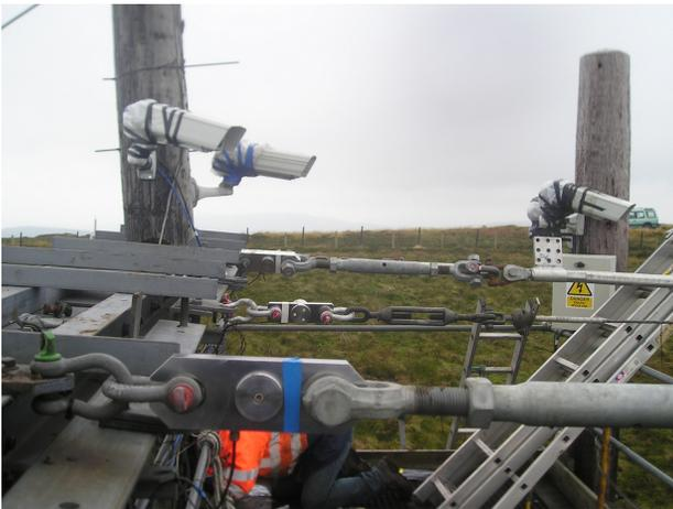
Fig. 3.2. The video cameras and load cells on the Southern H-pole on the Deadwater Fell test site.
